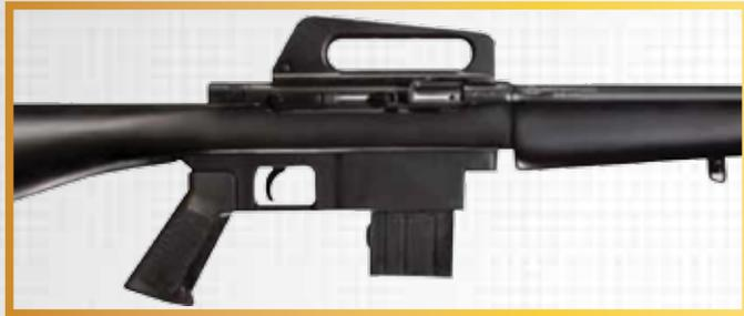
Draw safety on and insert a loaded magazine into the rifle. Retract bolt handle fully to the rear of the receiver slot and release. Allow the bolt to be snapped back under the full force of the operating springs. Bolt automatically picks up a cartridge from the magazine and feeds it into the chamber. Do not ease bolt forward.
