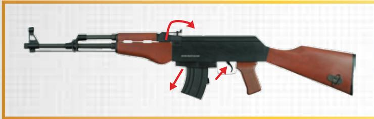
To unload your rifle, you must first detach magazine box from the rifle. Then, the chamber of the rifle can be cleared by holding the bolt handle and pulling it fully rearward (bolt open) and let it snap forward freely. This must be done repeatedly until the chamber is free of any cartridge.
