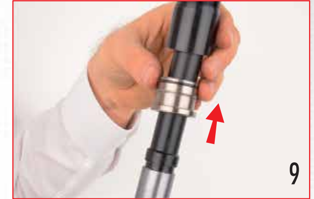
9) Remove the piston by pulling in arrow direction
