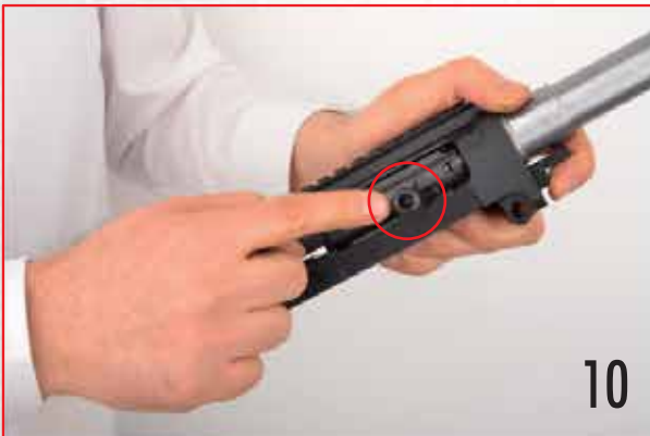
10) Remove the charging handle by pulling it
