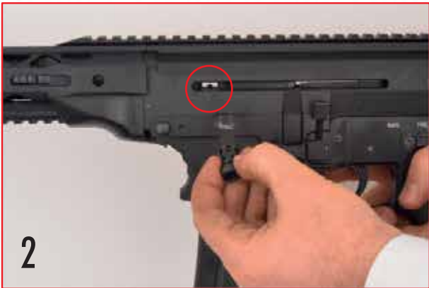
2) Insert the charging handle from the other side
