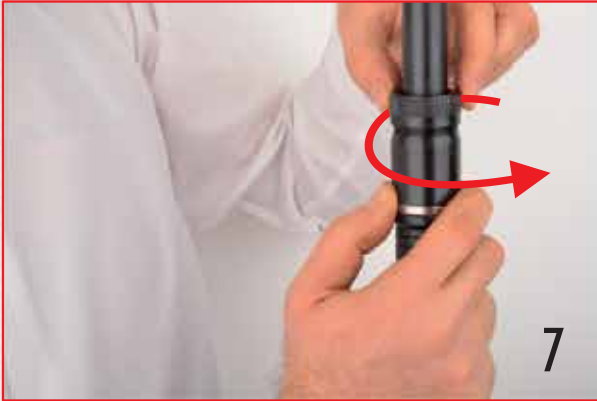
7) Unscrew the gas system retaining nut by turning in arrow direction
