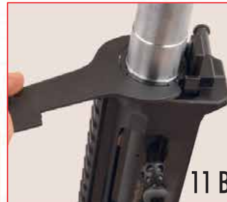
11A) Remove both barrel screws with a wrench 11B) Remove both barrel retaining rings with the MK12 multi tool
