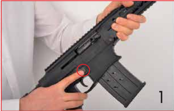
1) Remove the magazine
