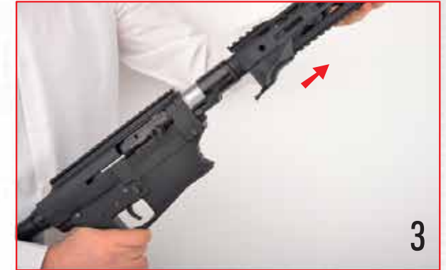
3) Pull the fore end in arrow direction
