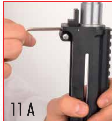
11A) Remove both barrel screws with a wrench 11B) Remove both barrel retaining rings with the MK12 multi tool
